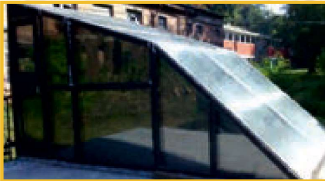
Head based storage Solar Kiln
